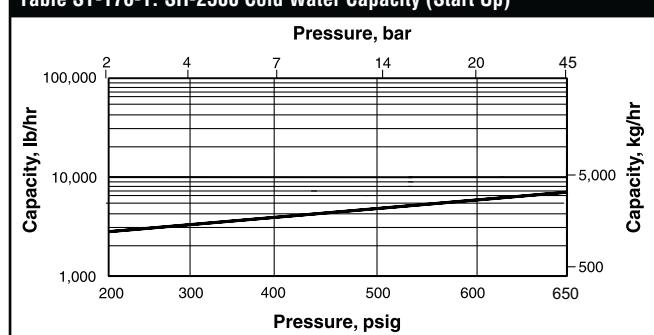
Note: Cold water capacity for start-up loads only. When superheat present, there will be minimal condensate.
