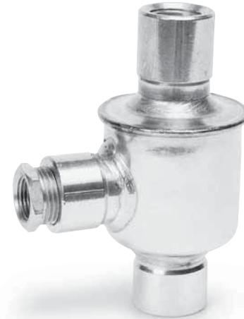
The Armstrong TAVB is a combination thermostatic air vent/vacuum breaker that is ideally suited for steam-filled vessels with modulating controls. The TAVB will vent air and other non-condensables from vessels such as shell and tube heat exchangers, jacketed kettles and steam coils during their operation. It will also break the vacuum that forms during steam control modulation.
